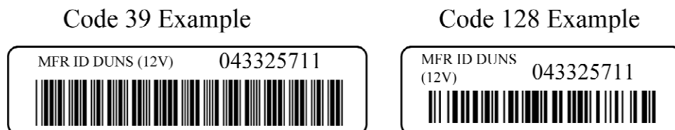
Figure F.1 — Example using DUNS Number in bar codes
