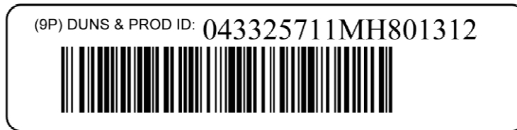
Figure FG.2 — Example using DUNS Number combined with product identification in bar codes
