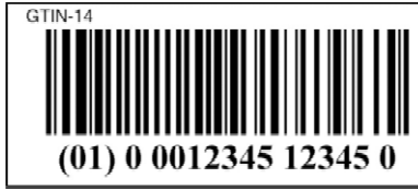
Figure 2 — Bar code symbol example with Application Identifier
