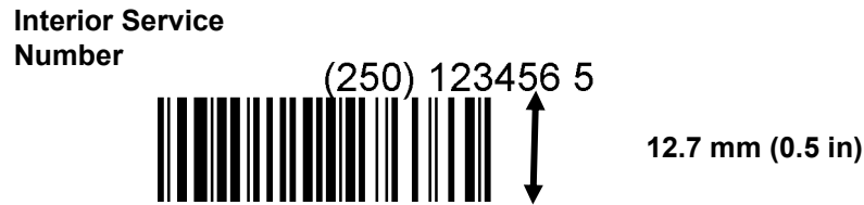
Figure H-6 – Resultant interior serial number
